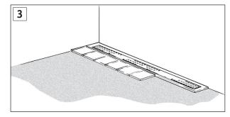
3. Lay the floor tiles with fall in one direction towards the channel.
