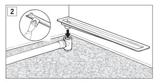
**2.** Install the drain in the water trap and embed in concrete.
