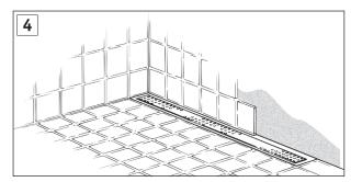
4. Fit the wall tiles leaving space at the bottom of the wall for a joint between tiles and frame.
