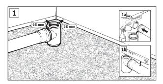
Embed the outlet pipe with water trap type 510.000. xxx in the structural concrete, placed in the left corner. Adjust the height as necessary.
