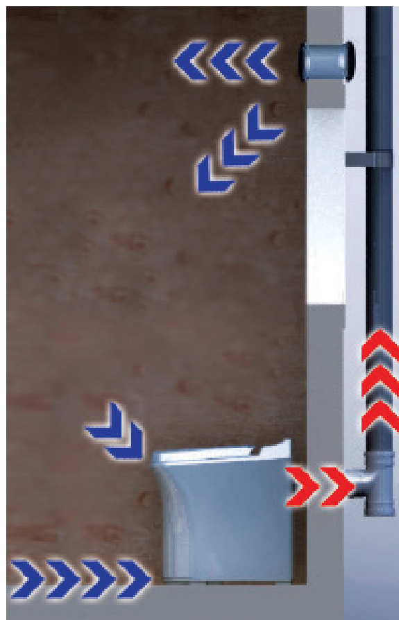
The toilet sucks in air from beneath the toilet and around the lid. Exhaust air ventilates through pipe in the wall.
